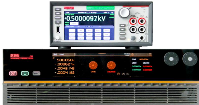
PVD measuring voltage vs. 6½ digit multi-meter
