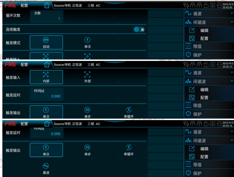
Figure 116 Interface of Interharmonic Configuration
