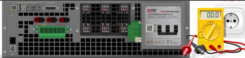
Figure 1. Schematic Diagram of Residual Voltage Check of AC Input Filter After Disconnecting AC Power
