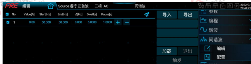
Figure 112 Interharmonic Parameter Setting Interface
