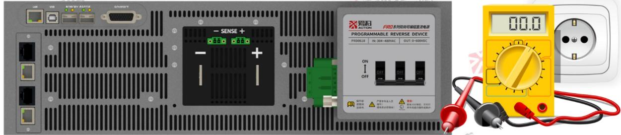
Figure 1-Power Port Residual Voltage Check Diagram
