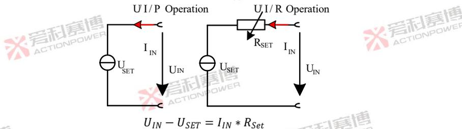
Figure 99- Constant Resistance Load Mode
