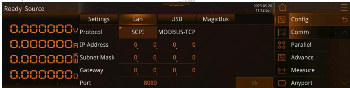
Figure 192-Config-Communication-Lan Screen
