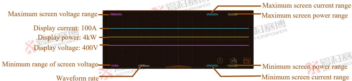
Figure 104-Waveform Reproduction Diagram
