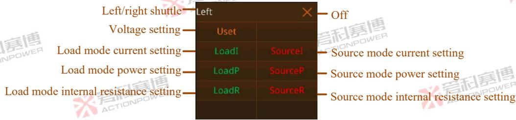
Figure 102-Shuttle Parameter Selection Screen
