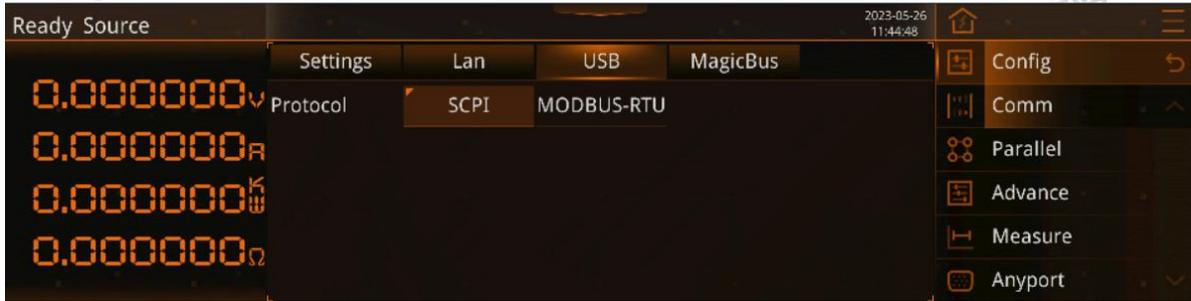
Figure 193-Config-Communication-USB Screen
