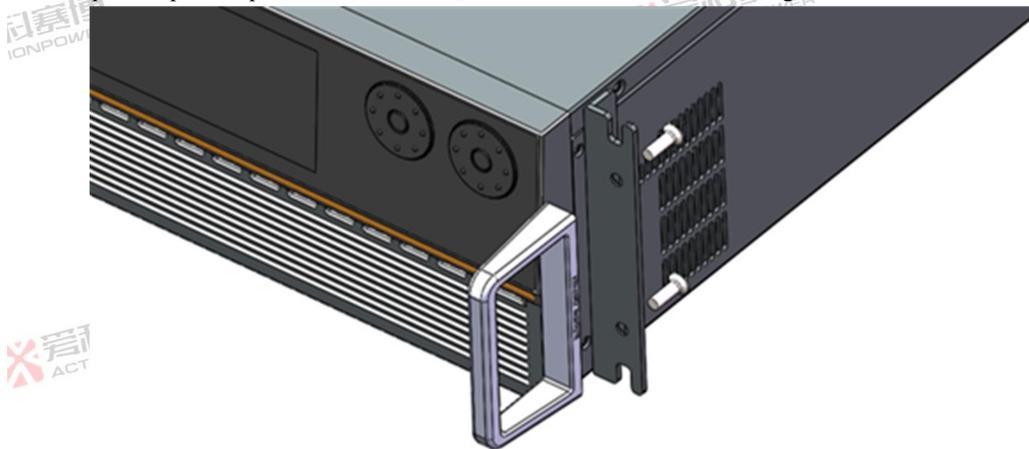
Figure 69-Handle Installation
