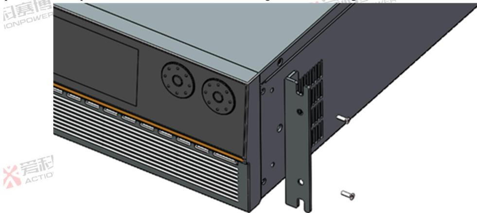
Figure 68-Hanger Installation
