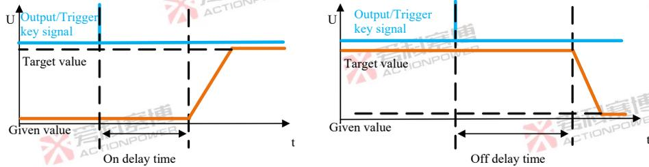
Figure 182-Output on or off delay time diagram
