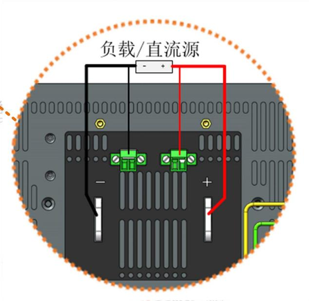
Figure 76-Remote Sensing Wiring
