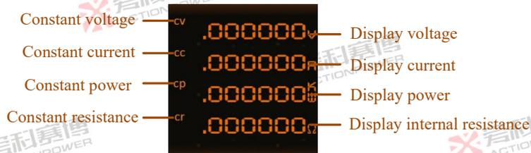
Figure 97-Output Display Screen
