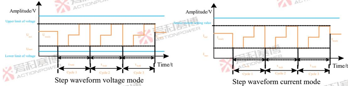
Figure 137-Step Configure Voltage/Current Mode Waveforms
