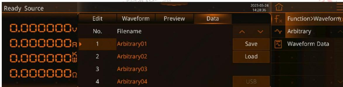
Figure 116-Function-Waveforms-Arbitrary Waveforms-Data Screen
