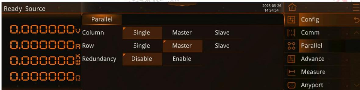
Figure 198-Line Parallel Master Config-Parallel Screen
