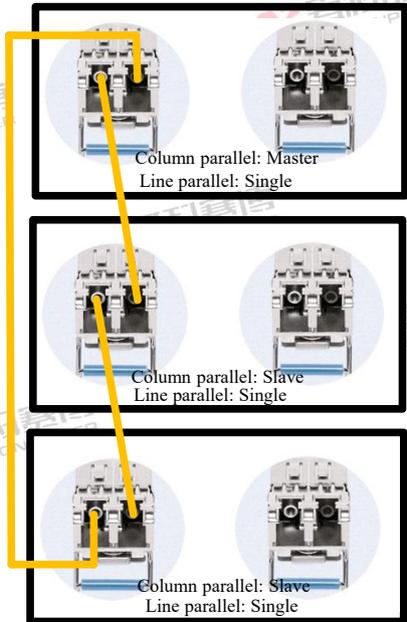
Figure 194-Column Parallel Optical Fiber Connection
