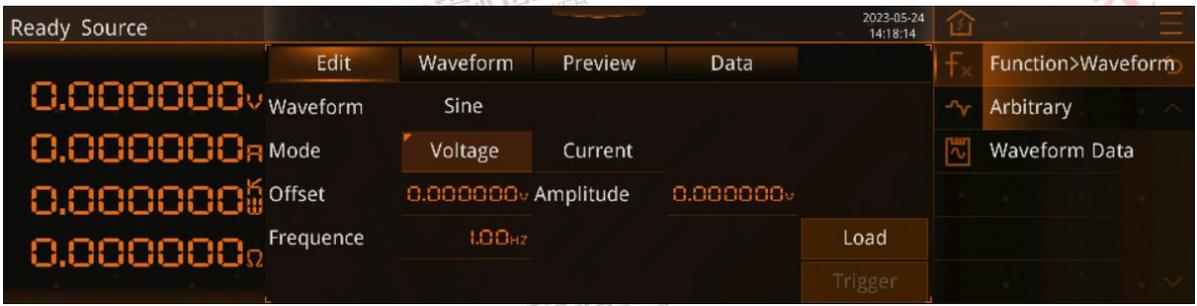
Figure 110-Arbitrary Waveforms-Edit Screen
