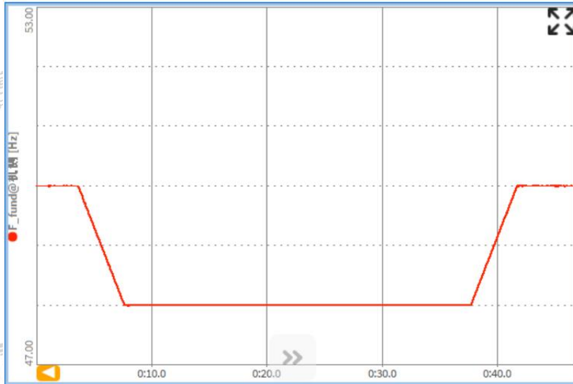
The output frequency is reduced from 50Hz to 48Hz and recovered after 30s
