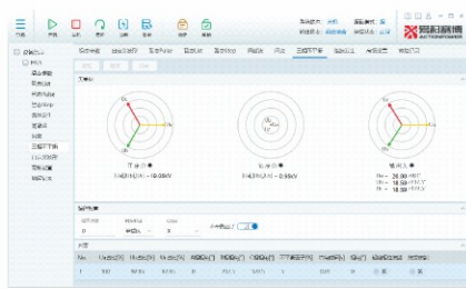
Three-phase unbalance setting interface
